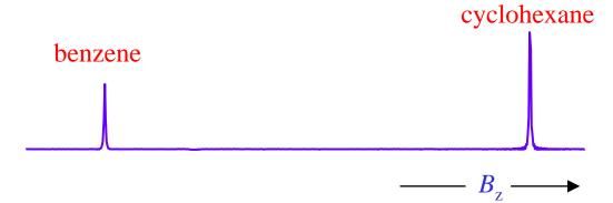
The spectrum is displayed as if for an increase in field, *but* differences in line positions are always quoted in frequency units.
