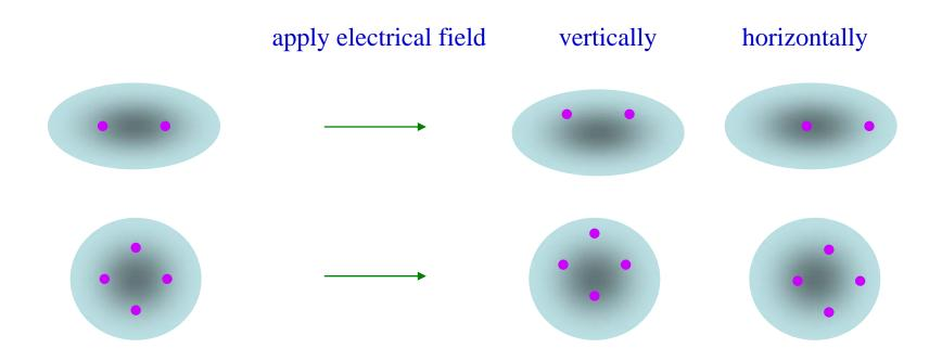
Rotational Spectrum:Raman active if the polarizability of the molecule is anisotropic.Spherically symmetric molecules are Raman inactive.
