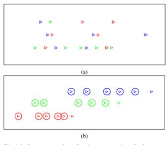
Fig. 10: System snapshots for three categories of robots: (a) Initial dispersion (b) Three lanes formed; one each for a group of like colours
