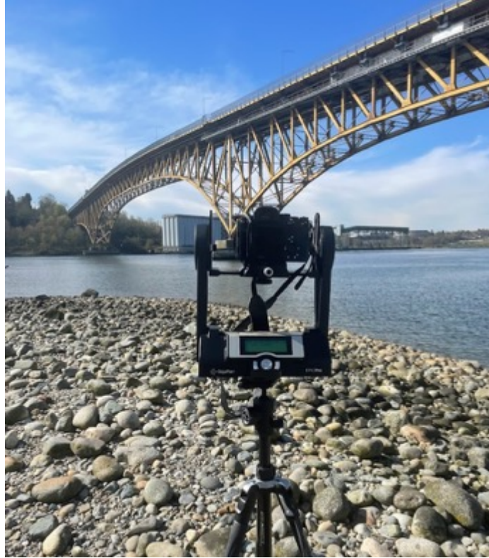
Figure 5. The GigaPan EpicPro with the Sony camera mounted on top in front of the IWMB, North Vancouver, British Columbia
