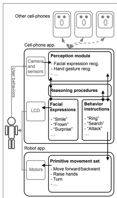
**Figure 3.** Implementation architecture of the proposed cell-phone robot
