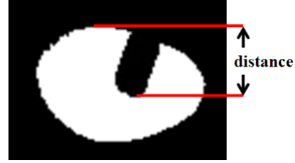
Figure 4. Distance between top of the pad's region and bottom of the stick.
